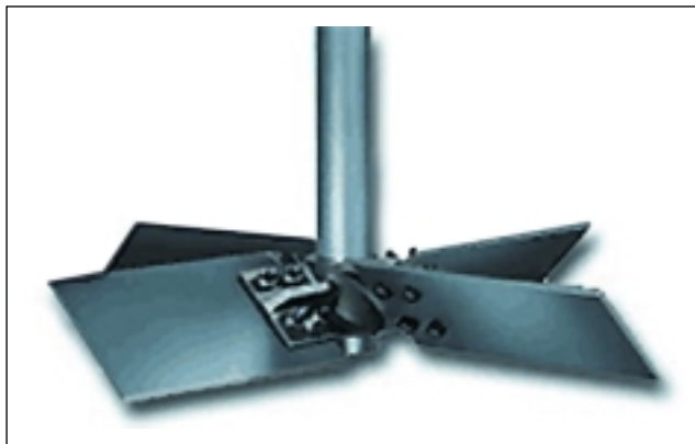
■ Figure 2. The pitched-blade turbine — a first-generation pitched-blade impeller — is used primarily for pumping. It has problems in gas-dispersion services because it allows gas bubbles to coalesce quickly. More recently, it has been replaced by hydrofoil axial-flow impellers. Photocredit: Chemineer, Inc.
