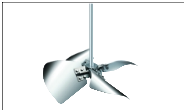
■ Figure 3. The high-solidity axial-flow impeller — a third-generation axial impeller — enhances axial mixing in a fermenter in the presence of very high gas flowrates. Photocredit: Chemineer, Inc.
