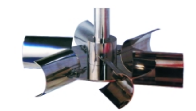
■ Figure 4. The concave-blade radial impeller — a second-generation radial impeller — is ideal for gas dispersion. With higher gas-handling capabilities and gas-loading characteristics than its predecessors, this impeller has been the subject of numerous design configurations that have produced even more efficient gas-dispersion impellers. Photocredit: Chemineer, Inc.
