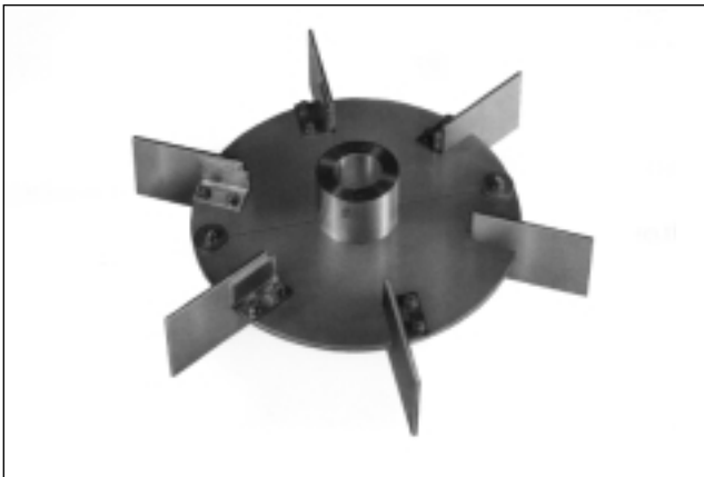
■ Figure 1. The Rushton turbine — a first-generation radial impeller — is used for gas dispersion. It has lower gas-handling and gas-loading characteristics than succeeding impellers in this family. Photocredit: Chemineer, Inc.
